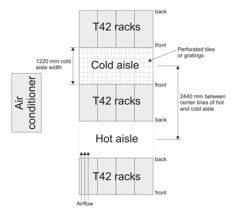
Figure 11. Example of cold aisle/hot aisle rack configuration
